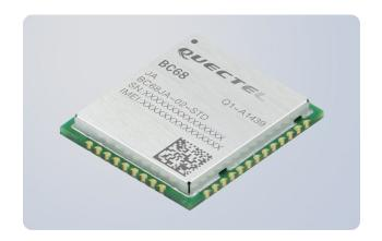
BC68 is a high-performance NB-IoT module which supports multiple frequency bands of B1/B3/B8/B5/B20/B28 with extremely low power consumption. The ultra-compact  $17.7 \, \text{mm} \times 15.8 \, \text{mm} \times 2.3 \, \text{mm}$  form factor makes it a perfect choice for size sensitive applications. Designed to be compatible with Quectel GSM/GPRS M66 module in the compact and unified form factor, it provides a flexible and scalable platform for migrating from GSM/GPRS to NB-IoT networks.
